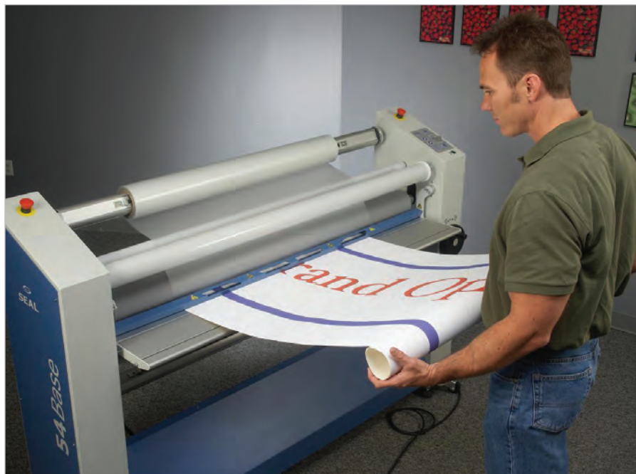
Try to use a laminating film that is the same width as your media, or one that is slightly narrower than your media sheet, but wider than the live area of the print. (Image courtesy of Neschen Americas)
