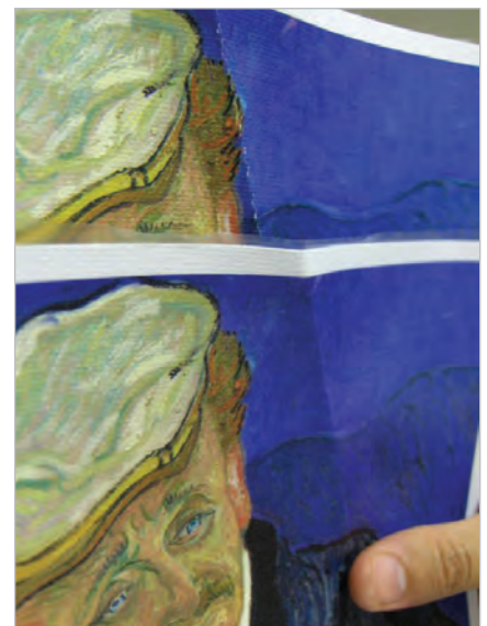
Sometimes clear coatings used on a giclée can crack when stretched over stretcher bars. An alternative is to dry mount a thin (2-mil) conformable clear protective film over the canvas image using a heated vacuum or dry-mount press. (Image courtesy of Drytac)
